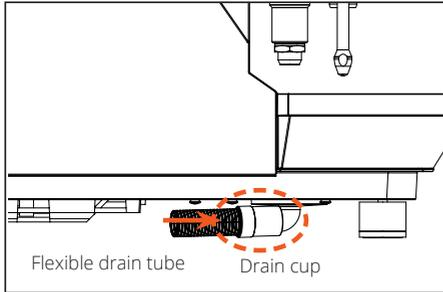
1. Connect one end of the flexible drain tube to the drain cup outlet. (It is located under the machine. Contact a service technician to do this task you are unsure how to access this area of the machine.)
