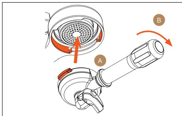
**A:** Align the portafilter's two flanges with the two slots in the group housing.
